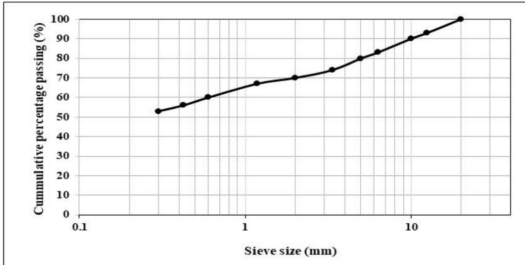
**Figure 1:** Particle size distribution curves of Laterite soil
