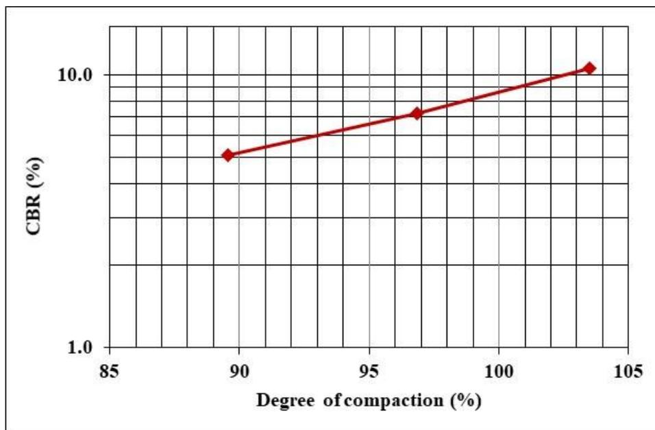
**Figure 3:** Three-point CBR values of Busale Laterite soil
