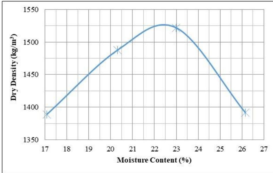
**Figure 2:** Compaction curve of the Laterite soil
