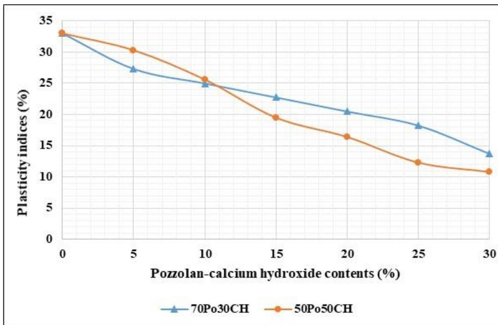
**Figure 4:** Plasticity index results for the stabilized Laterite soil sample
