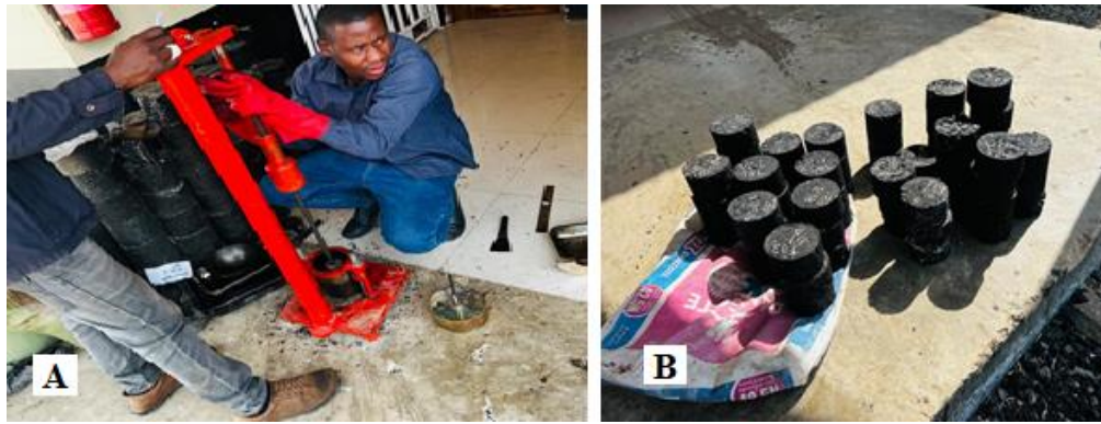
Figure A2: Photo for Marshall compaction process (A) and specimens (B)
