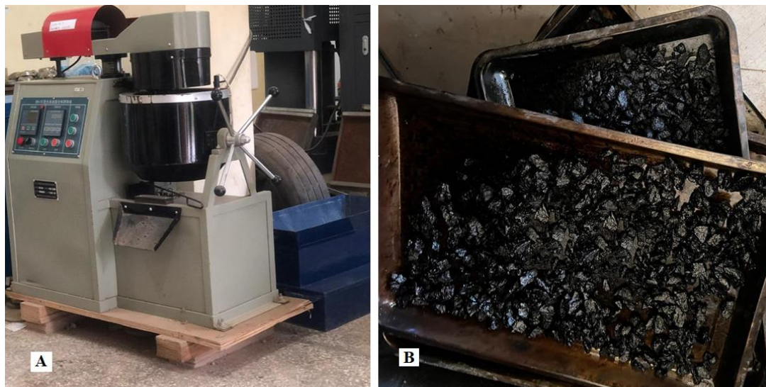
Figure 3: Asphalt concrete mixing machine (A) and loose asphalt concrete mixes (B)
